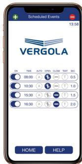
If you want the Vergola to chase the sun or shade at different times of the day and different times of the year, experiment with scheduled events to facilitate this functionality. The SEC function will facilitate the opening and/or closing of the Vergola in smaller or larger movements as per your preferences.
